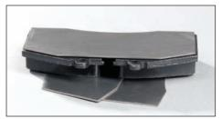
In racing applications, extreme measures are taken to keep heat out of the brake fluid. The shims shown above are fabricated from titanium, an excellent thermal insulator.
