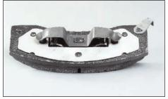
In order to reduce heat flow from the rotor to the brake fluid, a piece of insulating material can be placed between the backing plate and the caliper pistons. Stainless steel shims are the most common thermal barriers used in OEM applications and can also help to reduce certain noise frequencies. (Randall Shafer)
