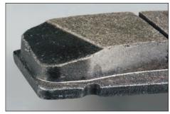
What differentiates one brake pad from another is the physical composition of its friction material. Like a fine suit, high-performance friction materials are custom-tailored to each application with a unique blend of ingredients. (Randall Shafer)
