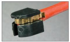
In some applications, a sensor is placed on the brake pad to alert the driver if the friction material is worn to its minimum thickness. While a spring on the backing plate can be used to emit an audible squeal under these conditions, the electronic sensor shown here informs the driver with a lamp on the instrument panel. (Randall Shafer/StopTech)
