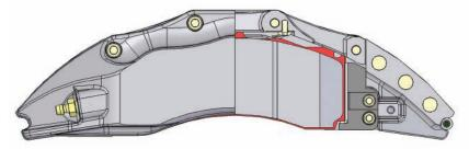
Caliper strength and stiffness are two key characteristics for optimum performance. Recent advances in computer modeling and simulation have allowed for significant improvements in both of these areas without the penalty of increased weight. (StopTech)
