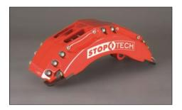
the hydraulic fluid pressure generated in the master cylinder into a linear mechanical clamping force against the brake pads. At the same time, the caliper will usually locate the brake pads and supports the torque generated by the brake rotor, but these are secondary functions.
