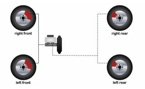
In a front-rear split design, the two front brakes (solid line) and two rear brakes (dashed line) use independent hydraulic circuits. This architecture is most common in rear-wheel drive vehicles and/or pickup trucks due to their significant rear weight distribution and large rear-brake assemblies.
