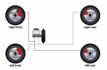
If a vehicle has a significant percentage of its weight carried on its front axle, the rear brake gain may be too low to achieve an appropriate level of deceleration during failed-circuit braking. For this reason, smaller vehicles with front-wheel drive typically employ a diagonally split hydraulic arrangement where the right front is paired with the left rear, and the left front is paired with the right rear.
