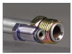
Smaller vehicles with smaller compliances require 3/16-inch brake lines as shown on the left, while large vehicles with excessive compliance require 3/8-inch diameter sewer pipes as shown on the right. If the brake line selected is too small in diameter, it will increase the brake system response time. (Randall Shafer)
