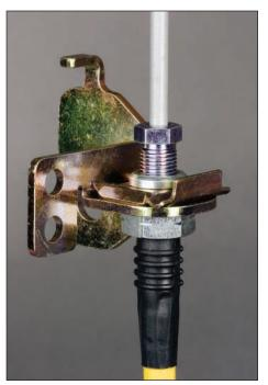
Because a brake line failure can be quite catastrophic, it makes sense to route them up and out of the way of any potential hazards. Clips and brackets should be used to attach individual lines to the vehicle body structure adding yet another layer of protection. (Randall Shafer/StopTech)
