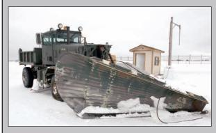
The overall brake system gain is a function of how much absolute force is required to stop the vehicle. Due to its weight, this 60,000-pound airport snowplow requires much more brake system gain than a typical passenger car. (Randall Shafer)
