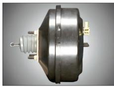
The gain of a brake system component is simply the relationship between the force coming in and the force going out. In the case of a brake booster, the ratio of these two forces is called the boost gain. (Randall Shafer)
