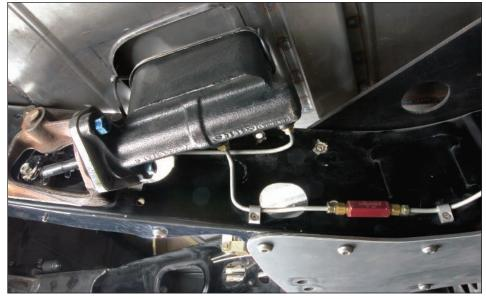
While the stock single-circuit master cylinder was swapped for a tandem unit, its location under the vehicle was retained. The tight confines dictated that an opening be cut in the floorpan to allow access to the brake fluid reservoir. Check out the elegant routing of the custom-bent brake lines! (Randall Shafer)
