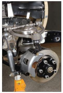
It took a significant amount of modification to adapt a Mustang II front suspension to the stock front frame rails. However, the front brake hardware remains essentially unchanged from the Mustang II design. Note that many hot rodders upgrade their Mustang II front end with a set of 11.0-inch diameter rotors and aftermarket caliper mounting brackets. (Randall Shafer)
