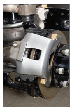
The Mustang II front brake calipers contain relatively large brake pads held in place by floating caliper bodies. The single piston in each caliper was designed to be offset relative to the center of the rotor friction disc, resulting in a larger effective radius. In plain English, this means higher gain is possible in a smaller package. (Randall Shafer)
