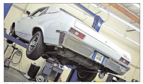
When this Chevy Nova was built in 1972, drum brakes had been replaced on most vehicles' front axles by disc brakes, but drums were still commonly found out back. Primarily because of their low cost, low weight, and superior parking brake performance, drums can still be found in modern rear brake applications where thermal requirements are low. (Baer)
