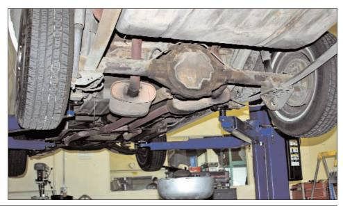
Nova was much more likely to see time at the drag strip than at the racetrack. Its front disc and rear drum brakes were common for vehicles of the era, and were relatively well-suited for boulevard cruising and sprinting from stop sign to stop sign. However, improved braking performance shouldn't be limited to vehicles with road course aspirations, and the owner of this particular vehicle had three distinct objectives in mind.
