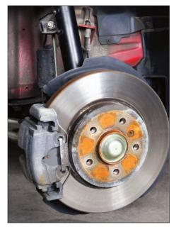
Removing the wheels and supporting the vehicle on suitable jack stands is usually the most safety-critical step in any brake system installation. Once you have the vehicle safely in the air, you have easy access to its stock brake system components. Regardless of which make and model you're working on, the stock front brakes probably look a lot like this. (Randall Shafer)
