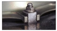
Since most rotor hat mounting methods allow for some unrestricted axial motion, they may rattle around when cold. Although not present on the racing rotor shown, anti-rattle springs are typically employed on street applications. (Randall Shafer)
