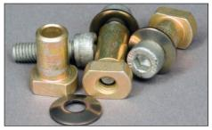
Two-piece rotors allow for relative movement between the friction disc and hat at temperature. Specialized fasteners are used to provide this freedom while simultaneously transmitting thousands of foot-pounds of brake torque. (Randall Shafer/StopTech)
