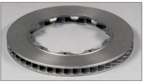
The friction disc is where all the action takes place. Because of its ideal mechanical properties and reasonable cost, gray cast iron is the predominant material of choice for nearly every friction disc today. The hazy film shown covering this friction disc is a coating to prevent corrosion before installation. (Randall Shafer/StopTech)
