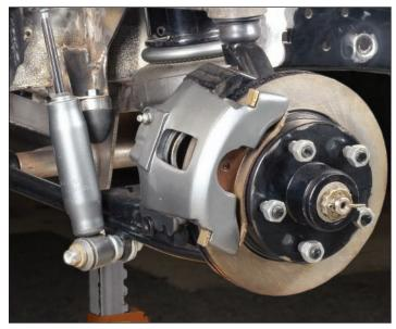
Although rotors are available in a variety of different shapes, sizes, and materials, they all share a common purpose—they must first absorb then dissipate a vehicle's kinetic energy during braking. While this rotor may be horribly undersized for a road racing application, it may fit the bill perfectly for a boulevard cruiser. (Randall Shafer)
