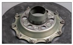
In the quest to further reduce rotating inertia, it's possible to use rotor hats made from exotic alloys. The hat shown above (already attached to a friction disc) was machined from a magnesium alloy. While cost prohibitive, it provides the lightest rotor assembly possible. (Randall Shafer)
