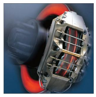
Regardless of their color, size, number of pistons, slots, holes, or sex appeal, the brakes don't stop the car. As you'll learn, they exist solely to convert energy from one form into another. A glowing rotor is a sure sign that the energy conversion process is in high gear. (Hawk Performance)
