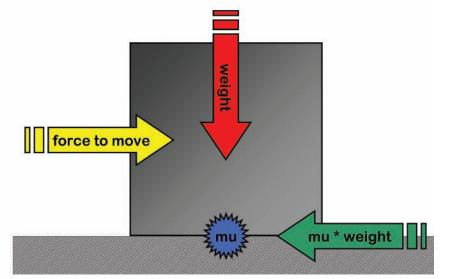
The force due to friction (green arrow) is equal to the coefficient of friction, or mu (blue star), multiplied by the object's weight (red arrow). This is equal to the force required to move the object along the surface (yellow arrow). As a result, the lower the coefficient of friction, the easier the object will be to move.
