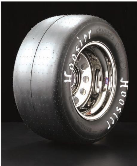
*The brakes don't stop the car—that's the tires' job! For this reason, tires come in a wide variety of shapes, sizes, and designs to optimize the available brake force. The lack of a tread pattern on this tire makes it a poor choice for wet-weather performance, but a great choice for racing when the track is dry. (Hoosier Racing Tire)*
