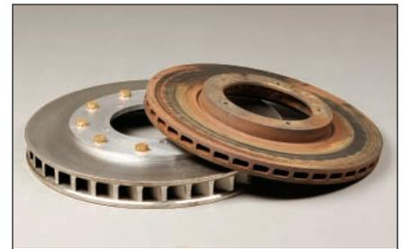
*The custom, two-piece front rotor shown on the left is 0.9 inches larger in diameter than the stock 911 rotor shown on the right, but even more impressive was the 0.5-inch growth in thickness. While thermal mass increased significantly (approximately five pounds per rotor), fabricating the hats from aluminum offset some of the rotational inertia impacts of the new rotors. (Randall Shafer)*
