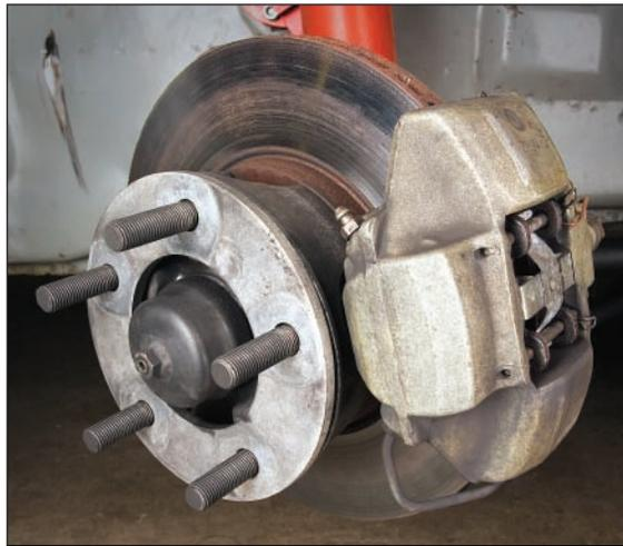
*Although it was world-class at the time, the stock 911 brake system from 1972 is only considered average by modern standards. Between the additional horsepower and modern race tires installed for competition, it didn't take many laps to realize the need for increased thermal capacity. The vintage brake systems found on Camaros, Corvettes, and Mustangs from the same era typically don't fare too well, either. (Randall Shafer)*
