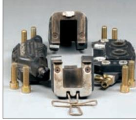
The basic caliper structure consists of body sections and bridge sections. In some applications, these may be discrete components assembled together. In the case of this early Porsche 911 Turbo caliper, two piston housings are bolted to two bridge sections to finalize the caliper assembly. (Randall Shafer)
