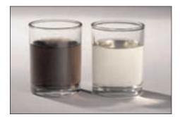
Time, temperature, and moisture are the three primary enemies of your vehicle's brake fluid. The only visual indication of degraded brake fluid performance is a change in fluid color over time from light yellow (the beaker on the right) to a dark, muddy brown (the beaker on the left). (Randall Shafer)
