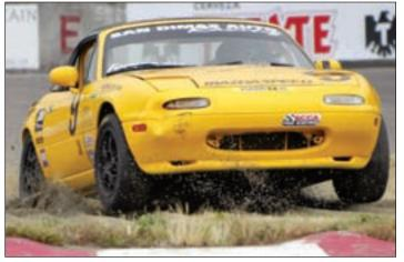
Brake fluid fade occurs when the brake fluid changes in state from a liquid to a gas. Unfortunately for the driver, brake fluid in vapor form is much more compressible than it is in liquid form, resulting in little, if any, braking effectiveness. Under these circumstances, the best one can hope for is a gravel trap to stop the car. (Wayne Flynn/pdxsports.com)
