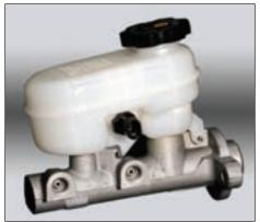
The brake fluid found in the master cylinder reservoir is not pressurized, even during brake application. This fluid is drawn into the hydraulic circuit only as needed due to long-term changes in brake system volumetric consumption, such as when brake pads are worn down to their backing plates. (Randall Shafer/Delphi Corporation)
