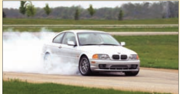
Tires generate brake forces through adhesive, deformation, and mechanical wearing modes of operation. Based on the surface, condition, and level of slip, a tire may be operating in one, two, or all three modes simultaneously. Tire smoke usually indicates too much mechanical wearing! (The Tire Rack)
