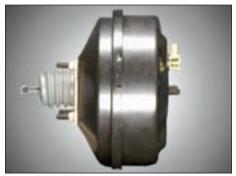
The gain of a brake system component is simply the relationship between the force coming in and the force going out. In the case of a brake booster, the ratio of these two forces is called the boost gain. (Randall Shafer)
